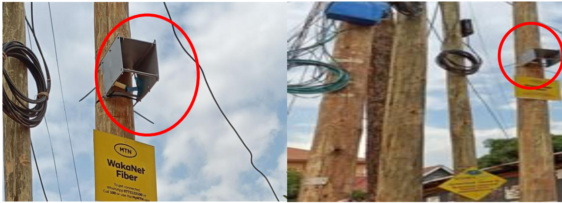
Figure 13: Deployed Air Quality Passive Samplers at the neighbourhoods of the proposed Code 4E Arua Aerodrome
