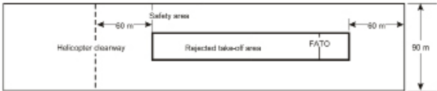
FIGURE S2-1. SAFETY AREA FOR INSTRUMENT FATO
