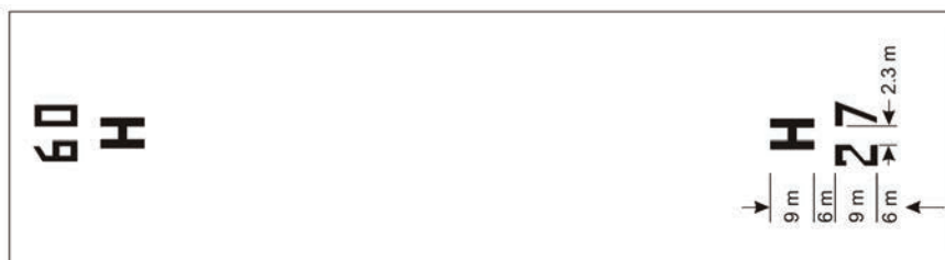
Figure 25: FATO designation marking and heliport identification marking for a runway type FATO
