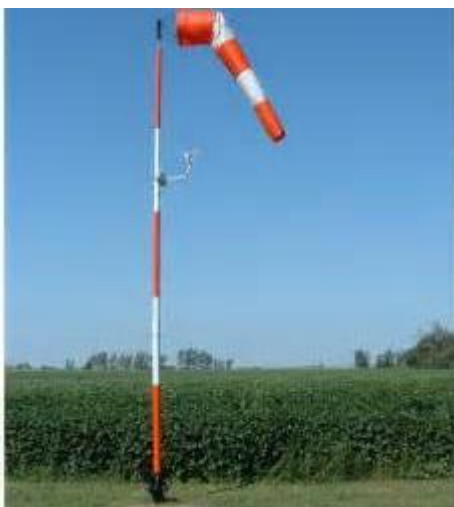
Figure 8: Sample marking of a wind direction indicator
