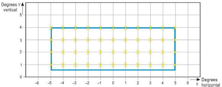
Figure S4-20. Isocandela diagram for high-intensity runway guard lights, Configuration B
